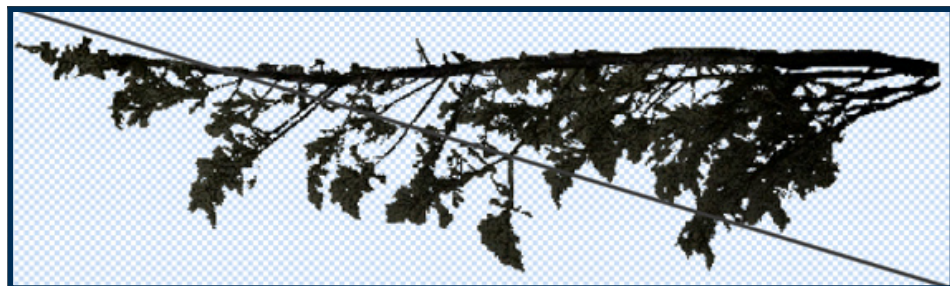
Figure 4. Example of a partially transparent leaf texture applied to a two-triangle surface.
